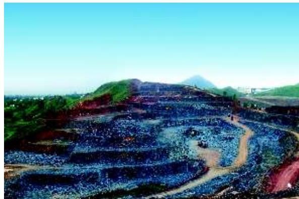
The first opencast uranium mine of the country at Banduhurang was commissioned in Jan. '09. Low grade mineralisation in this deposit continues to draw regular attention towards optimization of production and feed to the plant. The production capacity of this mine was augmented to 3500 tonnes per day.
